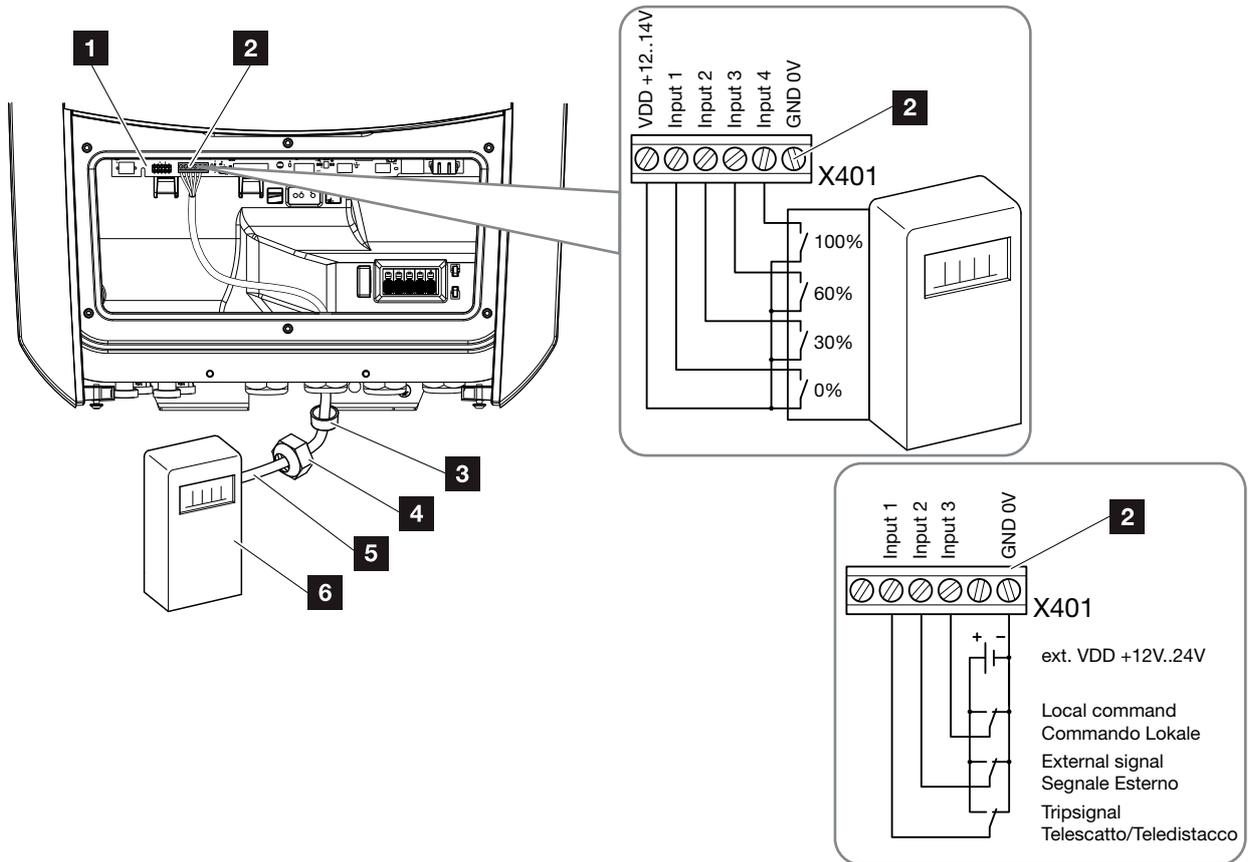
Abb. 31: Anschluss Rundsteuerempfänger
